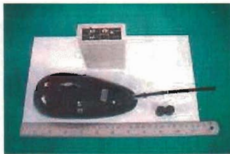
Fig. 2. Kiwisat101 manufactured by Sirtrack Ltd., weighs 600g with 1.0 w power.
